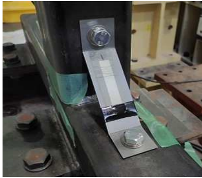
Figure 3. Setting of piezoelectric composite sensor.
